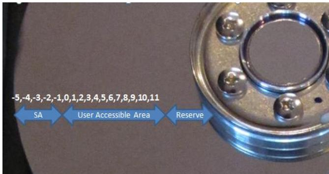
Figure 2 Sample Representation of a Hard Disk Drives Track layout
